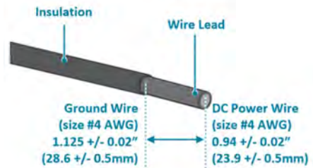
4-AWG green-and-yellow wire for grounding 4-AWG for DC power wire
